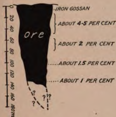
FIG. 41. — CROSS-SECTION OF RIO TINTO OREBODY, SHOWING DECREASE OF COPPER IN DEPTH. (VOGT)
